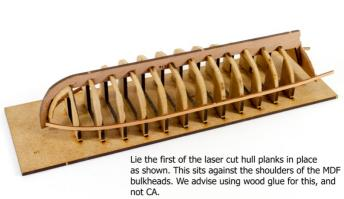
Note that the plank sits on the bulkheads with as much surface contact as possible due to previously bevelling the bulkheads
