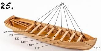
All of the seating now needs to be fitted, resting upon the seat support rails you fitted earlier. The seats are purposely over-length, allowing you to trim them specifically to your boat. With the seats in place, add the ribs (L30) from the 0.6mm pear wood sheet. Note they are doubled on the seats where the masts have support.
